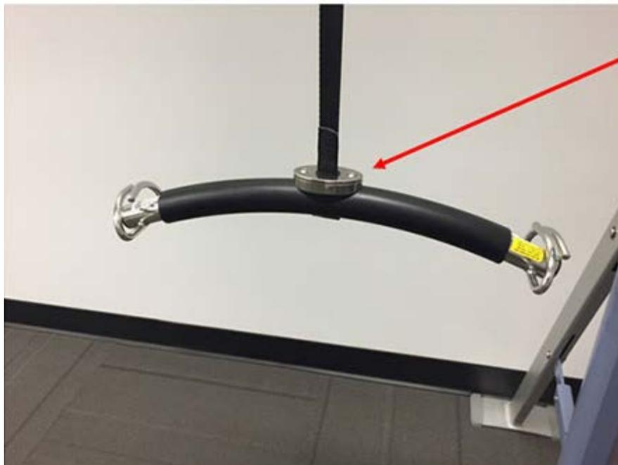
The 'puck' has a plastic swivel and attaches the strap to the carry bar.
