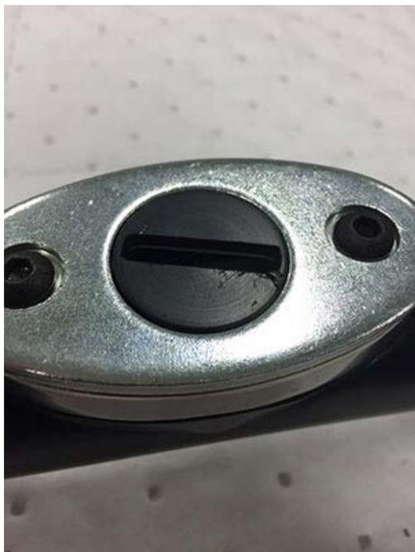
A 'puck' with a damaged plastic swivel. Look for any form of crack or divot or unusual widening of the opening.
