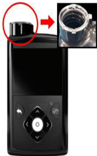
20 21 22 23 Image: Location of the retainer ring on the MiniMed™ 600 series insulin pump
